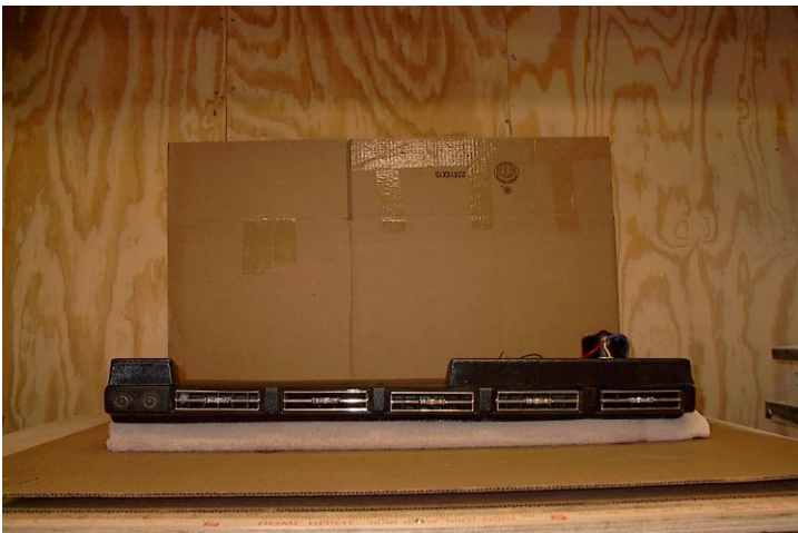
LHD Evaporator with Top Finish Panels Installed
