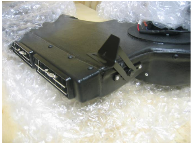
Custom Evaporator Bracket installed (1 Side)
