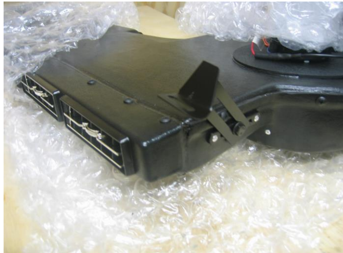
Custom Evaporator Bracket installed (1 Side)
