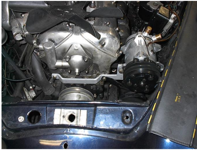
Same 3.8 Front Compressor Bracket on Mark II
